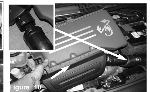
Figure 10 Now lift up and remove the air-box/engine cover from the vehicle. Disconnect the snorkel from the air box assembly.
