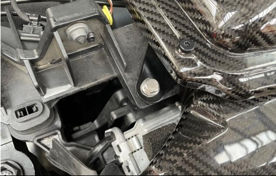
35. Secure remaining bracket with supplied M6 bolt. Bracket has been updated from the one shown.
