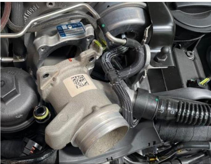
11. Remove the 3 Torx screws holding the right inlet in place. Remove the inlet and also remove the breather attachment – if your breather is connected to the inlet as shown here see next step. If you have the updated 2023 PCV breather system with the attachment to the top of the turbo please skip to step 12b.
