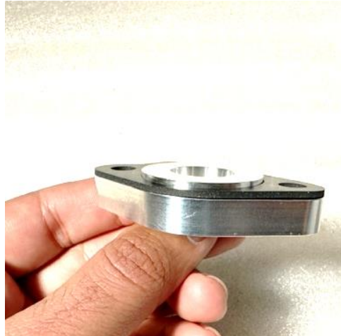
45. The gasket goes on the face with the raised central section. This goes onto the turbo with the gasket side facing down over the PCV opening.
