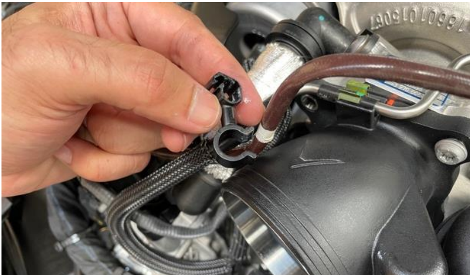
19. Remove the clip around the brown wiring sheath.
