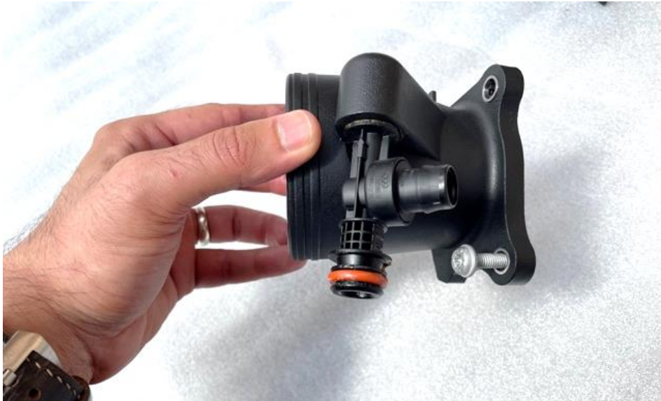
17. Push the breather into the left side inlet as far as possible. Green O-ring goes into the inlet. Also take one of the OEM screws and push it into the bottom hole as shown.
