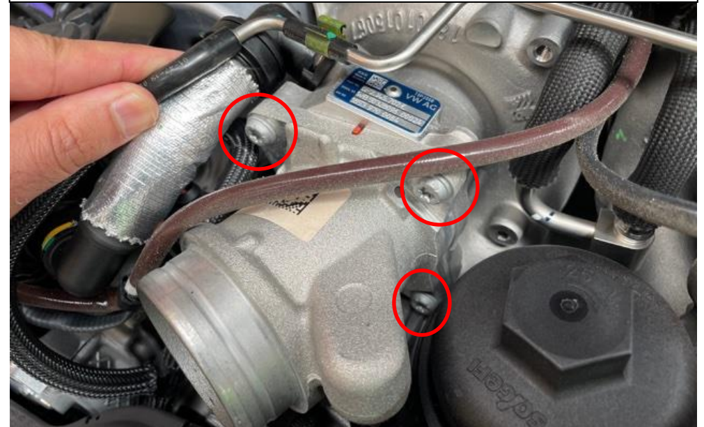
8. Remove the 3 Torx screws on the left side turbo inlet. The lower one can be accessed easier by removing the breather - see next step.
