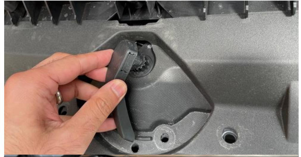
6. Remove the Hood release lever. There is a push clip on the side which needs to be pressed in order to release it.
