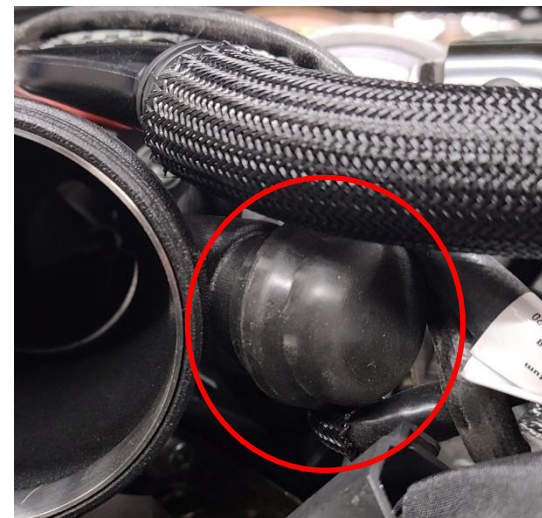
47. Ensure the rubber plug is blanking the breather port on the new inlet. Now go back to step 26 to complete the installation.
