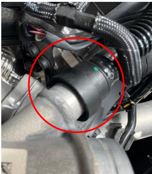
12. This breather attachment is secured with small internal clips. Use a small screwdriver or pick to push the clips back in order to release the tube from the inlet.
