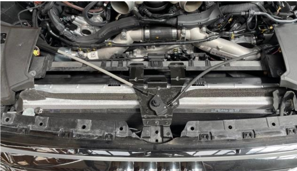
7. Now both the airbox base and the slam panel can be removed.
