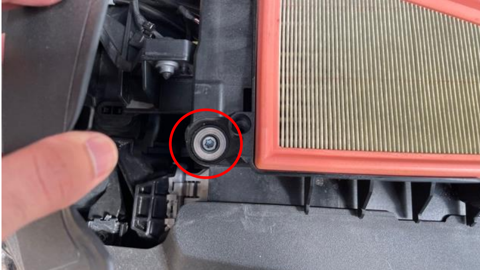
5. Unscrew the Torx screws on each side of the airbox.
