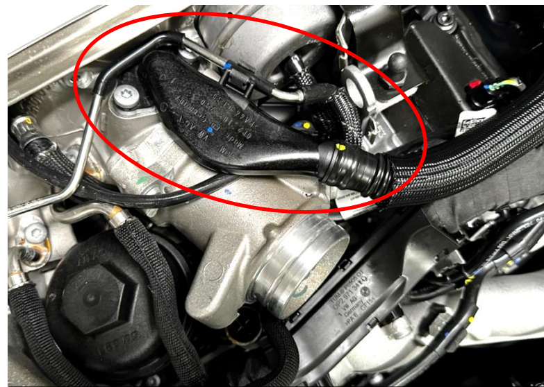
12b. If your breather is attached to the turbo as shown – remove the 2 torx screws holding it down to the turbo and remove for access to the inlet. Remove the inlet and follow the next steps. There is a spacer included to be used when reinstalling this breather for clearance over the new inlet.
