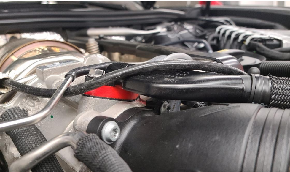
46. With the spacer in position (shown here in red) – refit the PCV breather on top of the spacer. Make sure the green O-ring in the breather is still in place when installing. Use the supplied M6 Torx screws to tighten the breather over the spacer.
