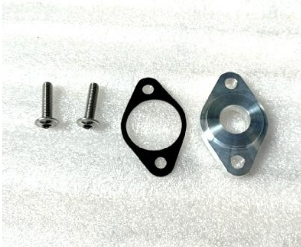
44. Please follow these steps if you have the 2023 updated PCV breather system. Take the spacer, gasket and 2 x M6 Torx screws from the kit.
