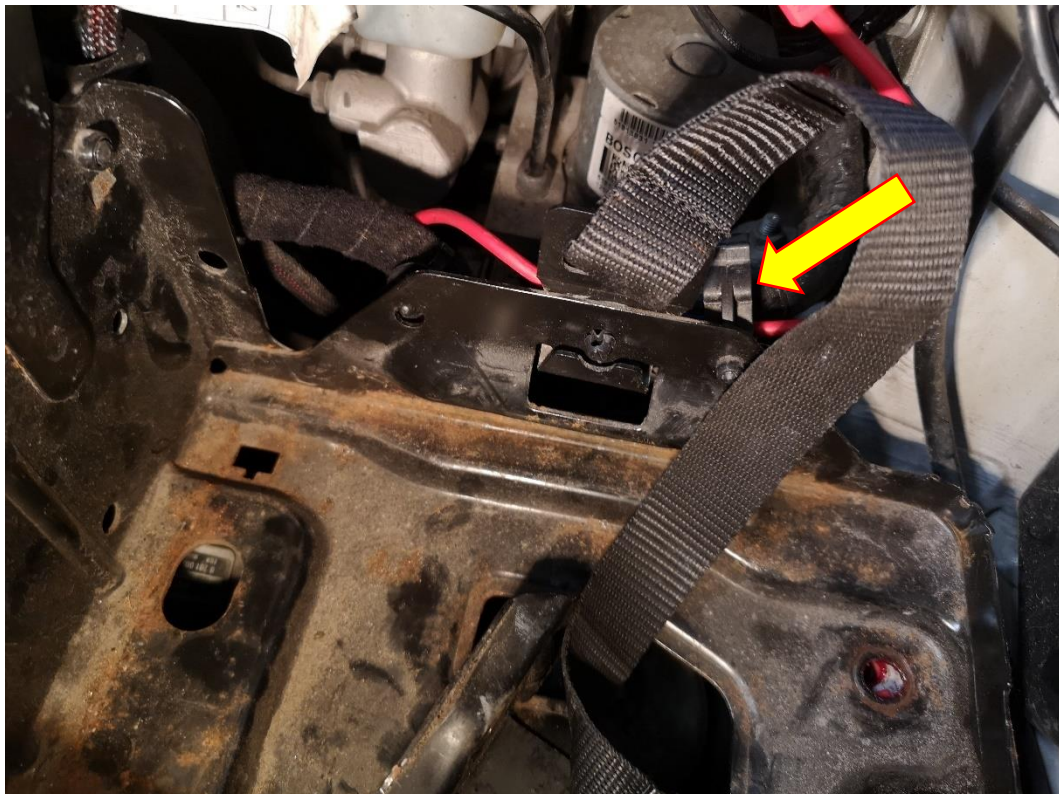
WIRING HARNESS CLIP THAT IS CONNECTED TO BATTERY STRAP BRACKET (X1)
